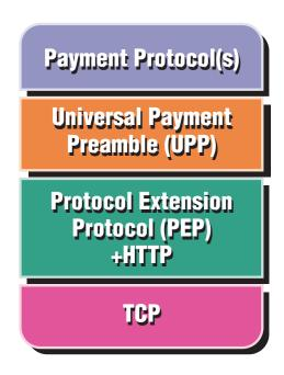
cation. The Universal Payment Preamble (UPP) is used to negotiate the payment protocol that will be used, based on the vagaries of each individual transaction. The negotiation itself is conducted in clear-text; any necessary security is provided by the payment protocol being used.
